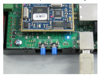
• On the IP7-MZC-FD, the reset pins are located behind the Primary Ethernet 10/100 connector
